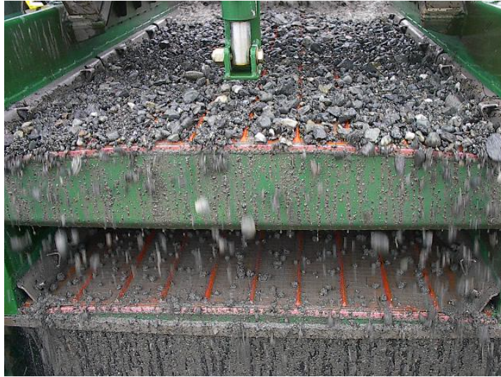
Figure 2. Crushed Rock from the Coarse Shaker Screen of the Soil Separation Plant
