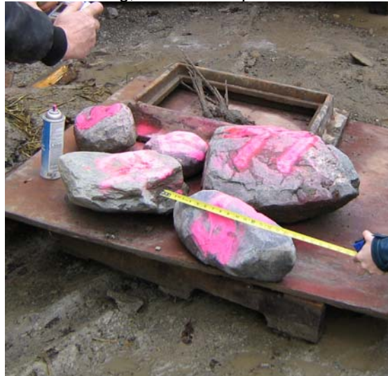
Figure 1. Boulders collected by the contractor during shaft excavation.
