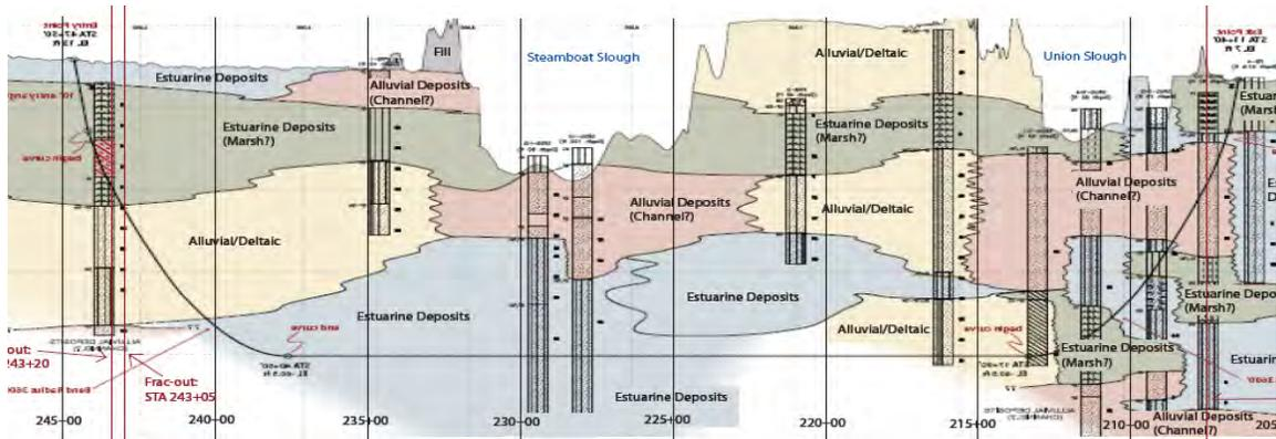
**Figure 4. Geotechnical Cross Section for the 5-South Crossing**
