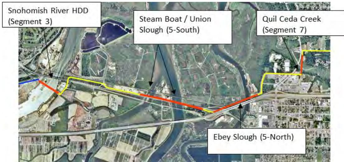
**Figure 2. HDD Bore Locations Relative to Entire Pipeline**
