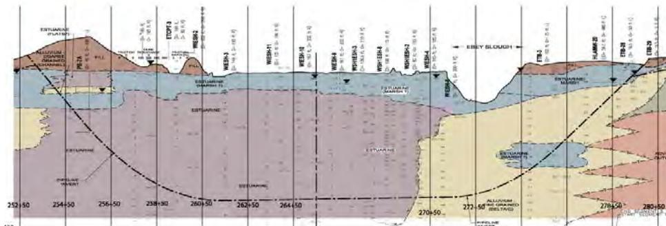
**Figure 3. Geotechnical Cross Section for the 5-North Crossing**
