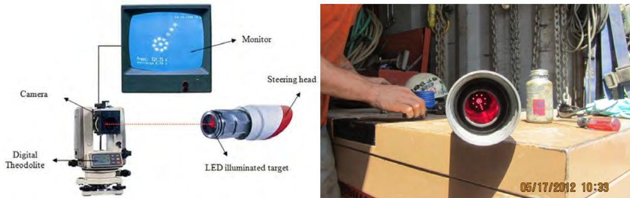
Figure 1. Pilot tube guidance system (left) and LED illuminated target (right).
