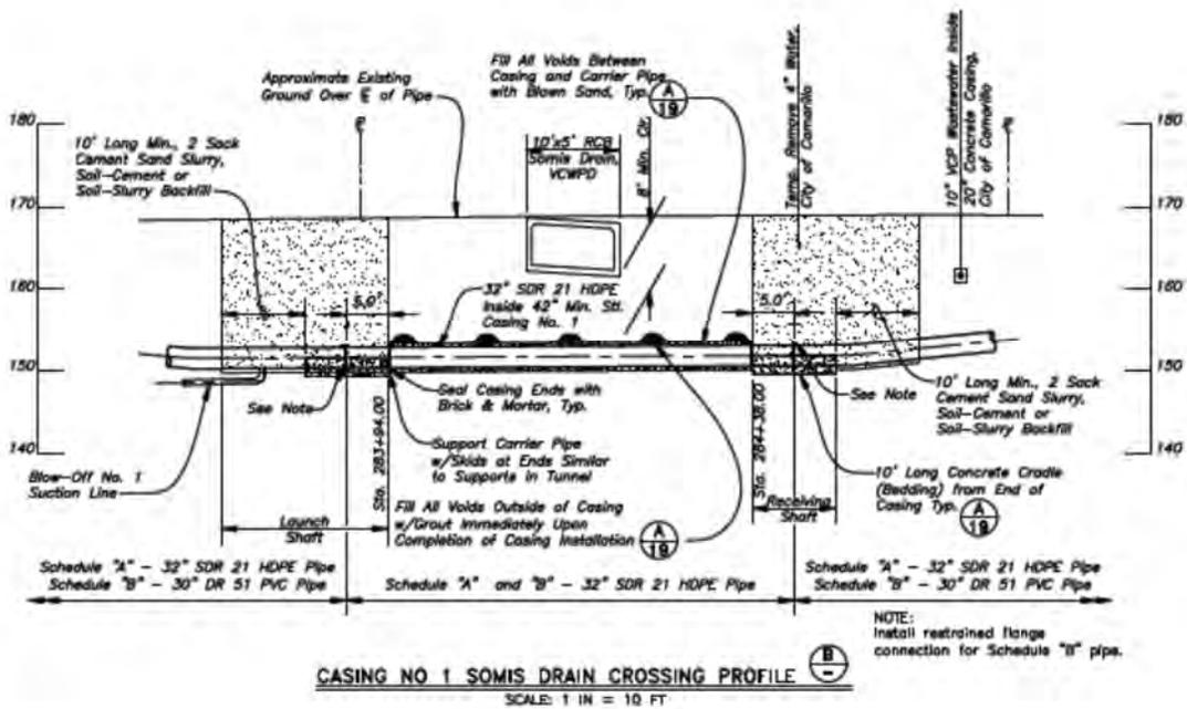
Figure 7. Profile view of the Somis Drain Crossing.
