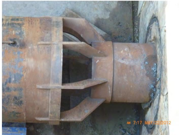
Figure 6. Forty two-inch reaming head installed behind the intermediate 24-inch casing.
