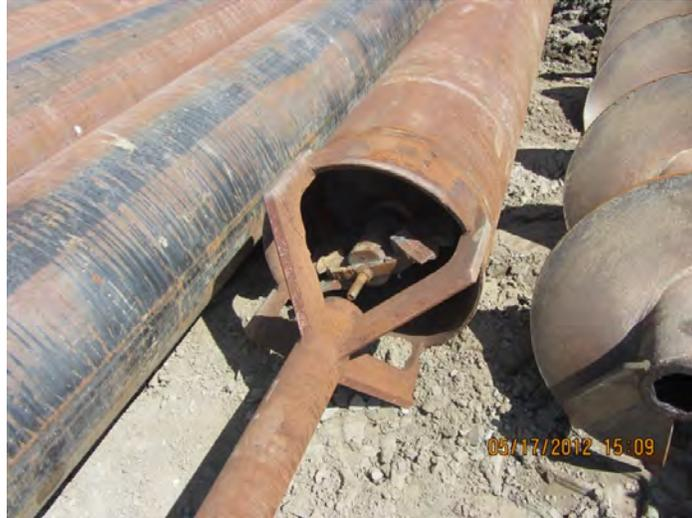
Figure 4. Twenty four-inch “reaming head” with adaptor tube.
