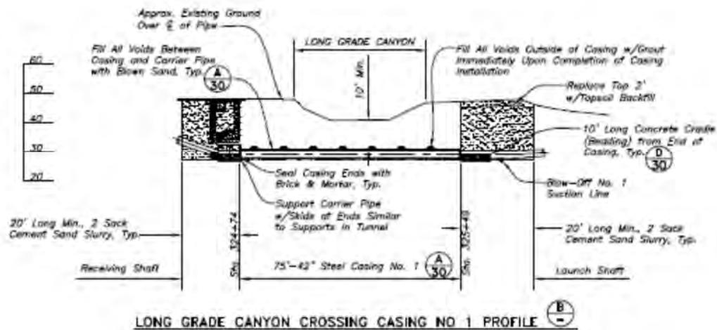
Figure 3. Profile view of the Long Grade Canyon Crossing.
