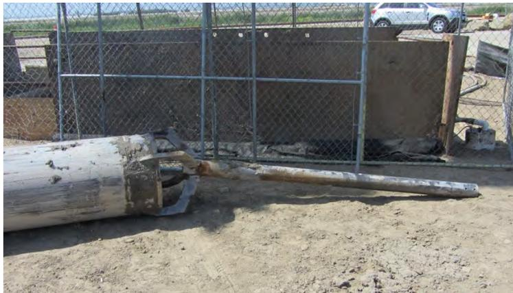
Figure 5. Bent adapter tube in front of the 24-inch reaming head after removal from the reception shaft.
