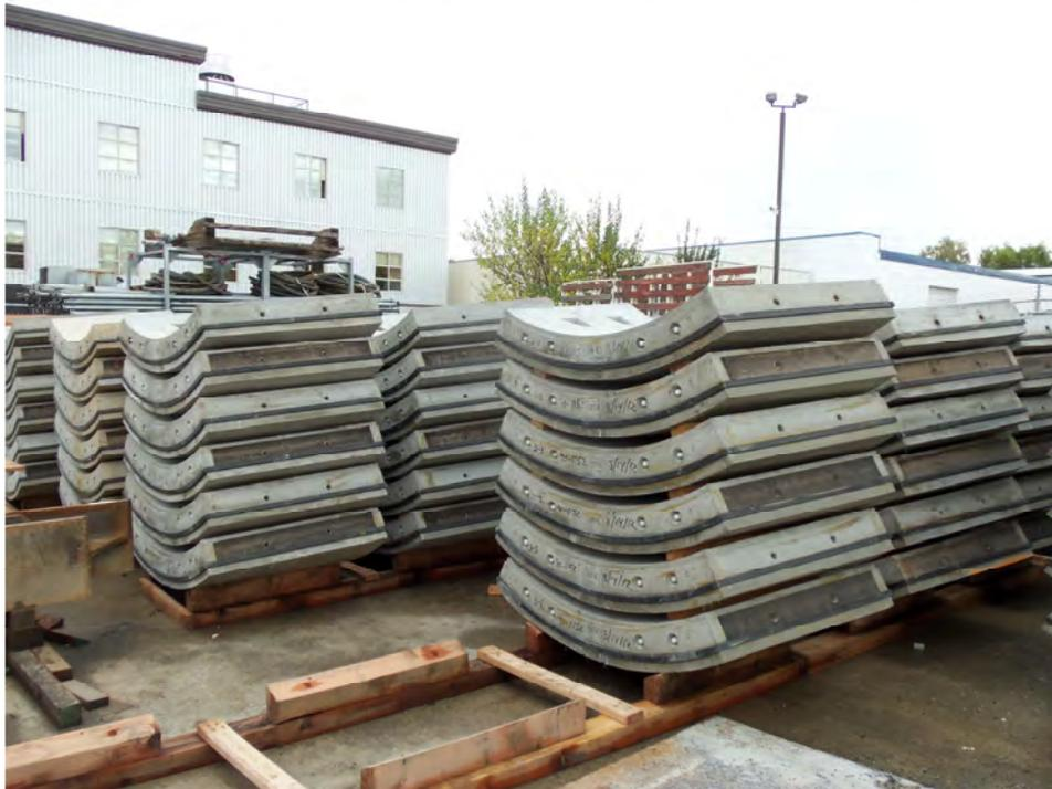
**Figure 5. Tunnel Segments used as the Initial Lining**
