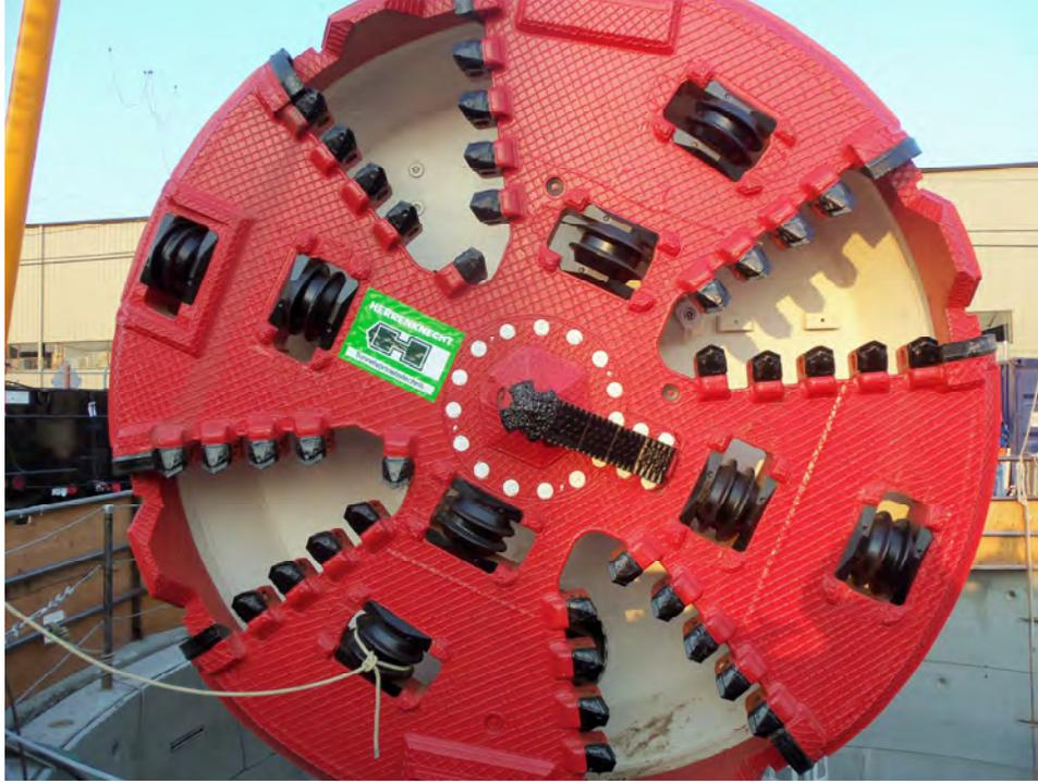
**Figure 3. EPBM Used for Excavating Beneath the Ship Canal**
