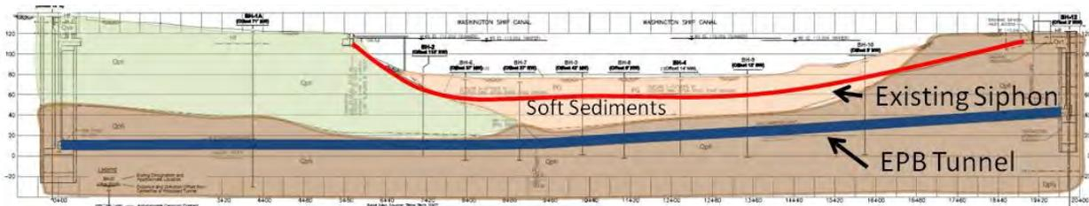
Figure 2. Geotechnical Cross Section
