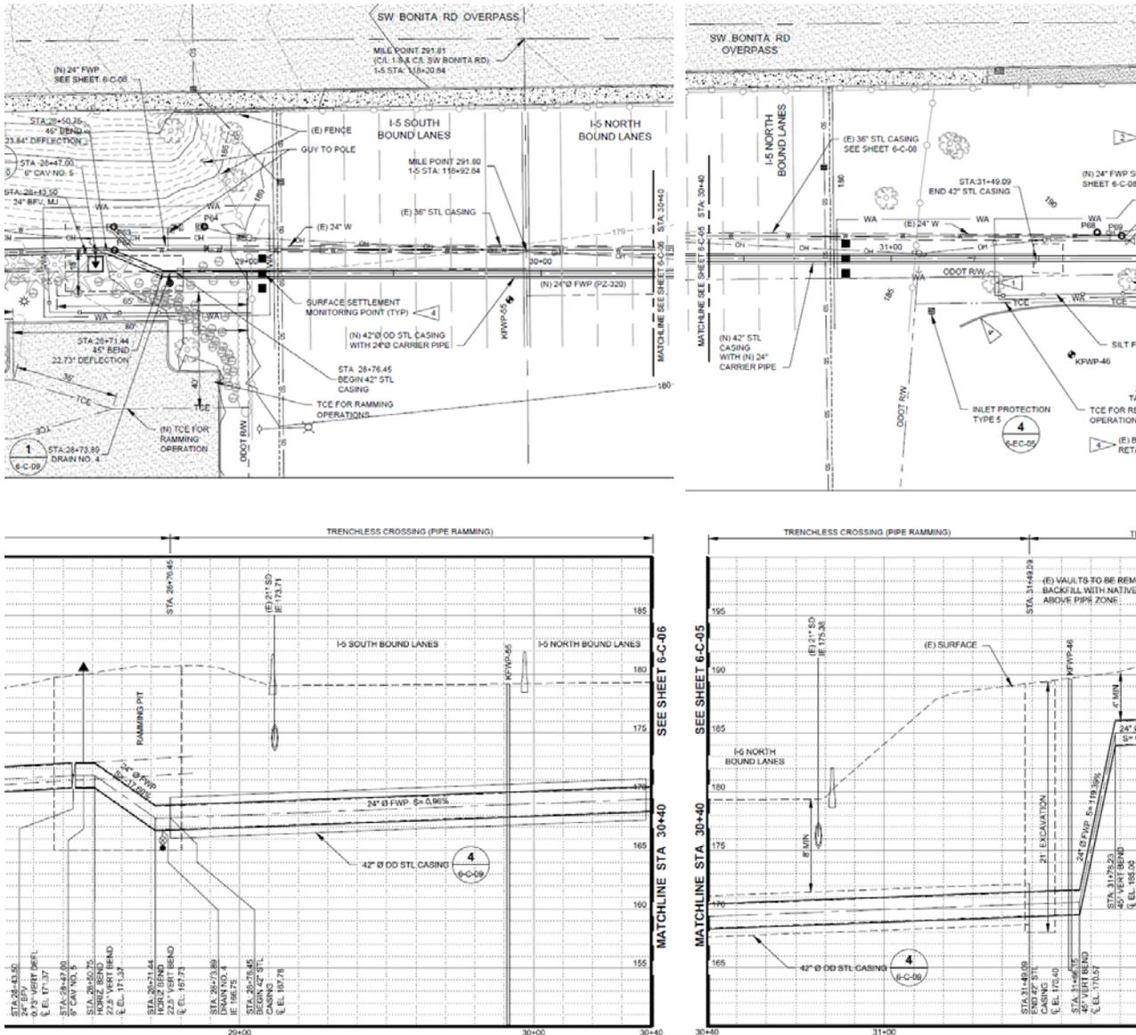
Figure 3: Finished Water Pipeline undercrossing of Interstate 5 (Tigard, Oregon)
