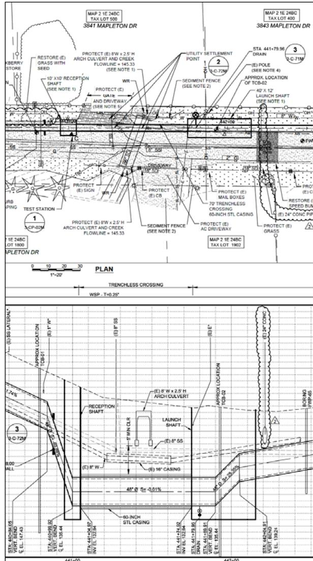
Figure 2: Finished Water Pipeline undercrossing of Trillium Creek (West Linn, Oregon)
