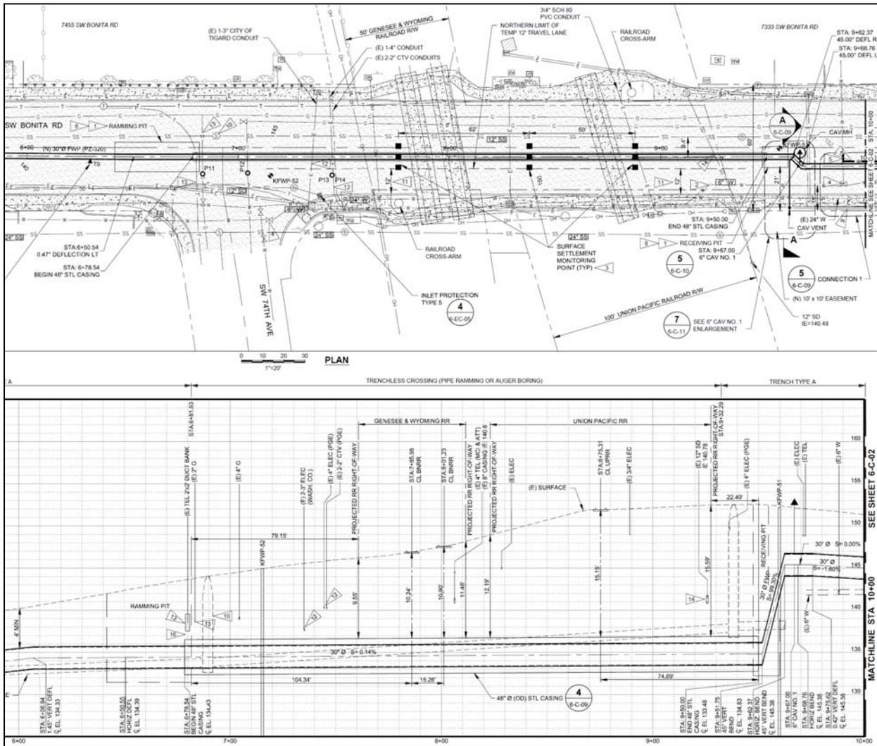
Figure 4: Finished Water Pipeline undercrossing of railroads (Bonita Road, Tigard, Oregon)
