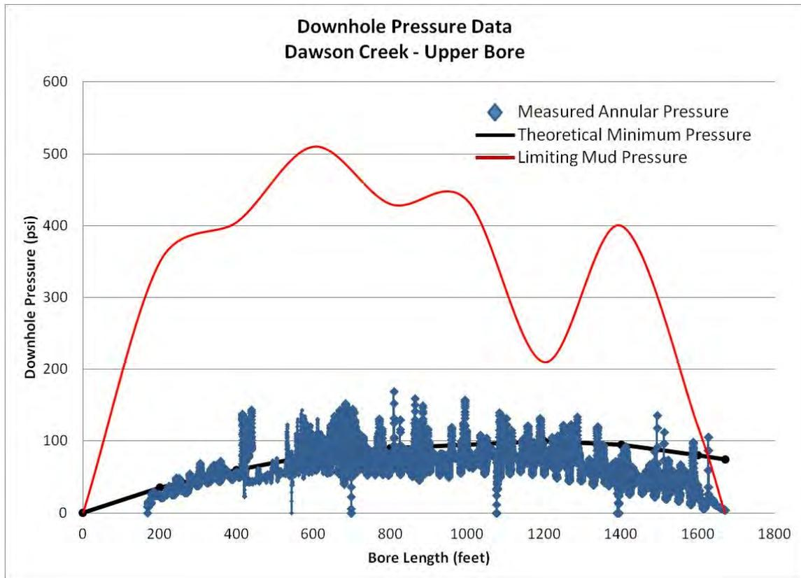
**Figure 8. Measured Annular Pressure- Pilot bore – Dawson Creek upper Bore**
