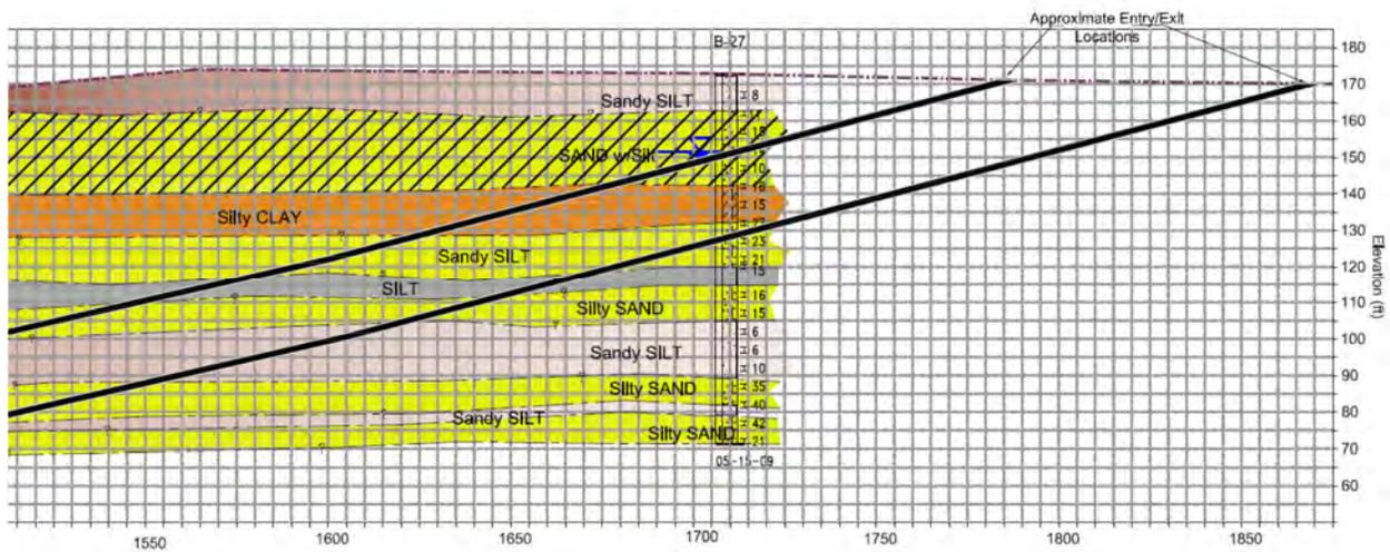
**Figure 4. Geology at the exit location with layered sands and silts.**
