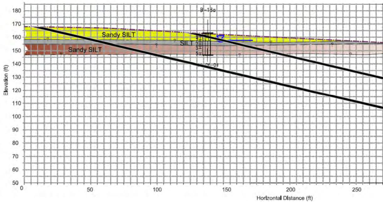
**Figure 3 Entry Location of the bores with the Geotechnical Information**
