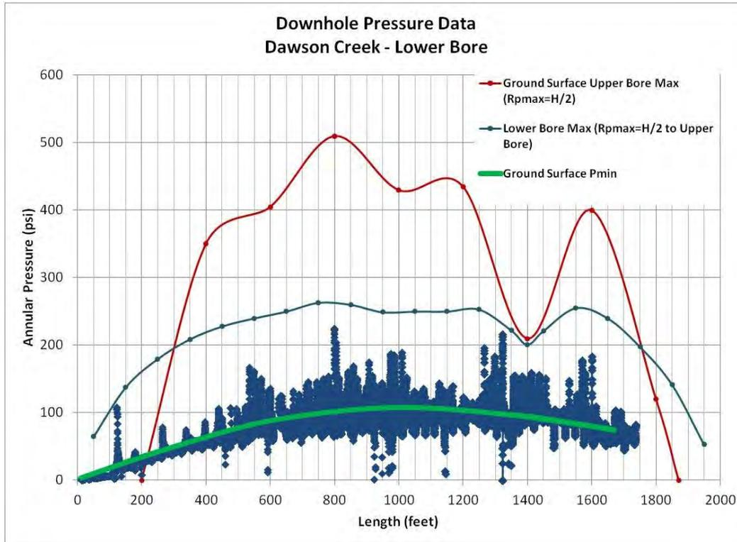
Figure 9. Measured Annular Pressure- Pilot bore – Dawson Creek Lower Bore
