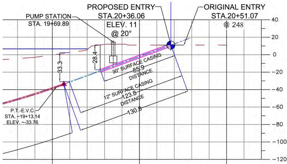
Figure 4. Contractor's Approved Entry Side Profile with Wet Well Pump and Conductor Casings.
