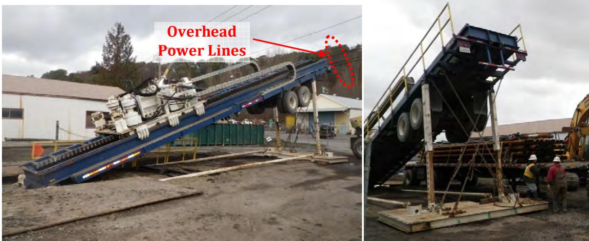
Figure 7. Drill rig setup at 20 degrees.
