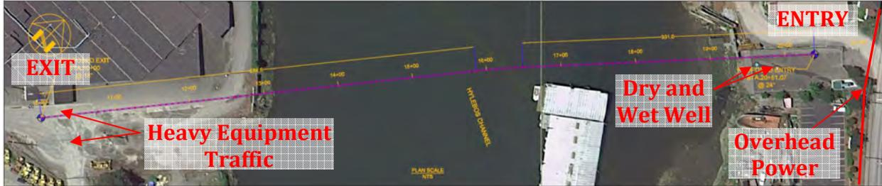
Figure 2. Plan View of the Hylebos Channel HDD Crossing
