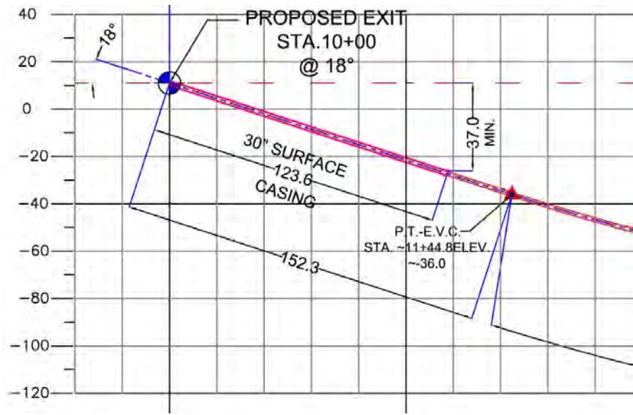
Figure 5. Exit Side Profile with Conductor Casing.
