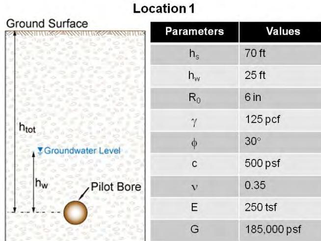
Figure 4. Location 1 - Geometry and Soil Parameters
