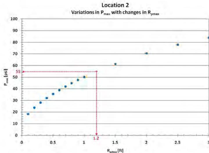
Figure 9. Location 2 Frac-out Pressure and Plastic Zone Radius
