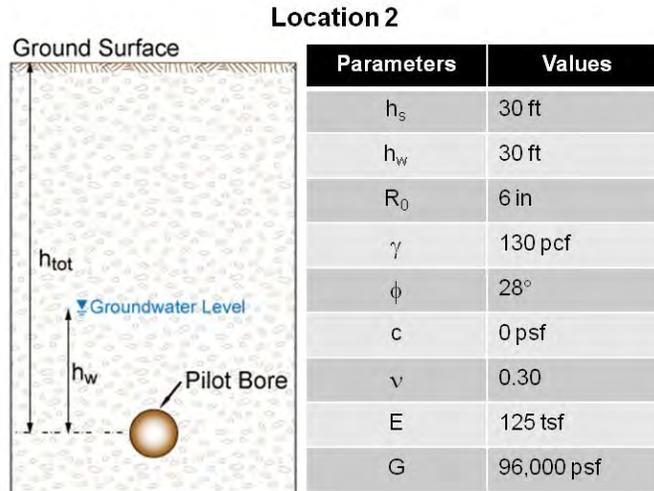
Figure 6. Location 2 - Geometry and Soil Parameters
