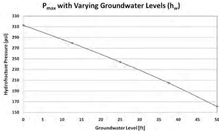
Figure 2. Effects of Changes in Groundwater Level on P<sub>max</sub>
