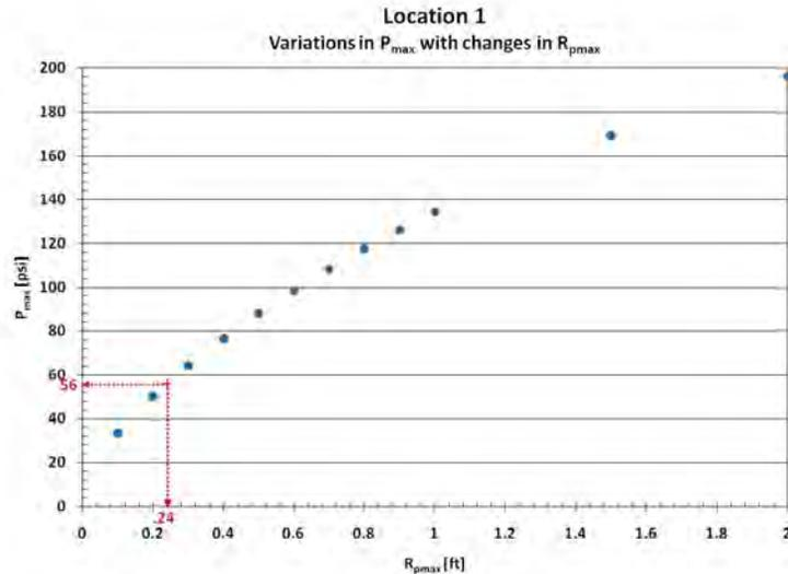
Figure 8. Location 1 Frac-out Pressure and Plastic Zone Radius
