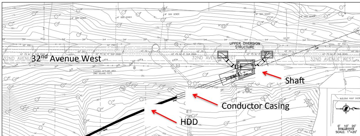
Figure 4. Location of Shaft on 32<sup>nd</sup> Avenue West (upper end of bore)
