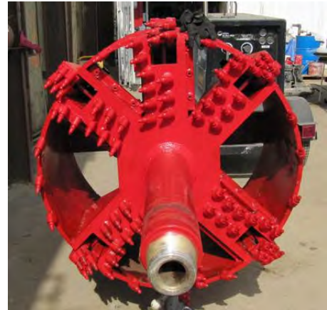
Figure 8. 45-inch reamer with expanding teeth
