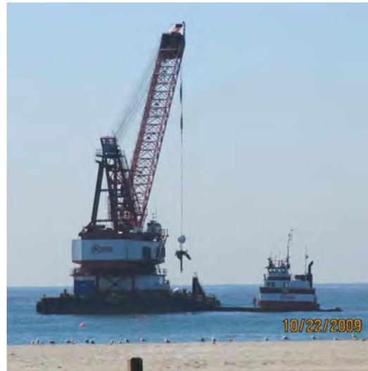
**Figure 6. Derrick barge and supporting tugboat from shore**
