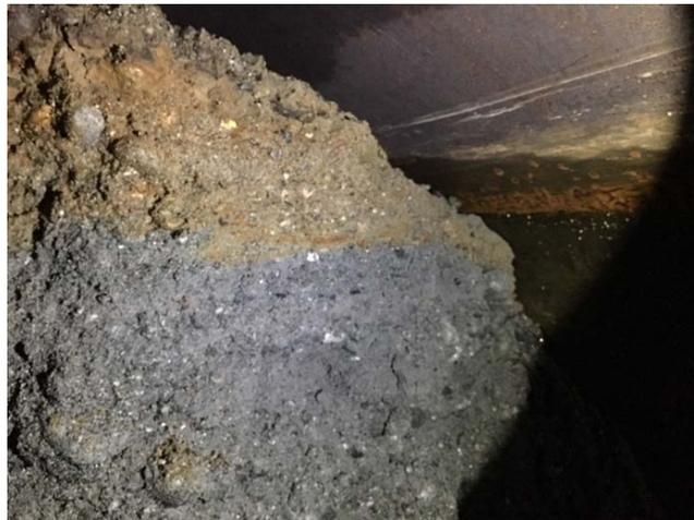
**Figure 9 Soil inside leading pipe segment showing alluvium/recessional soils (brown) underlain by dense glacially overridden soils (gray).**
