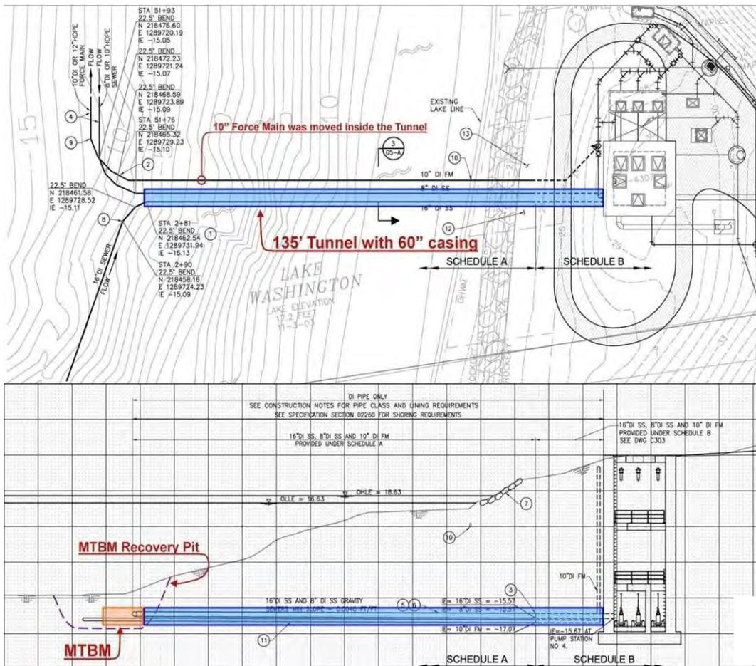
Figure 3. Contractor's Proposed Microtunnel
