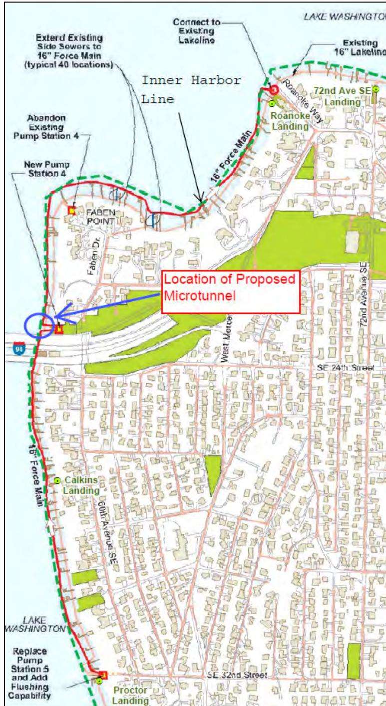
Figure 1. Existing Lake Line, New Lake Line, and Microtunnel Location
