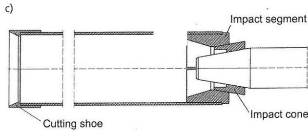
Figure 5. Pipe Ramming Setup (Stein, 2005)
