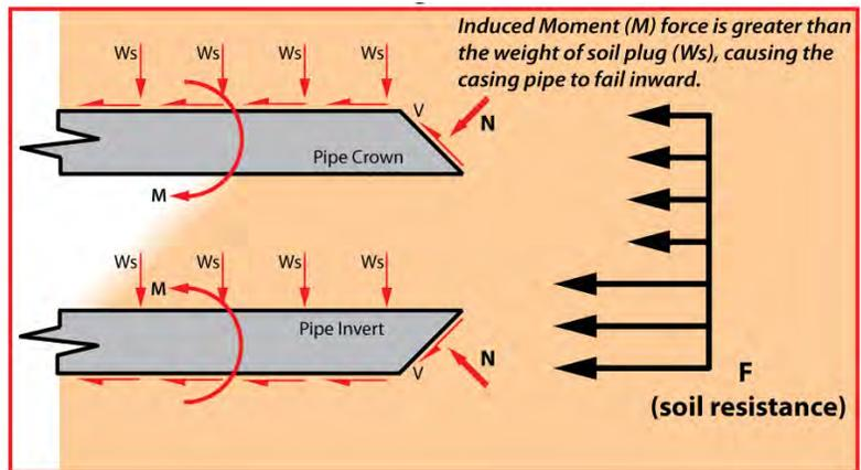
Figure 8. Force Diagram of Improperly Designed Cutting Shoe that Can Lead to Pipe Failure.
