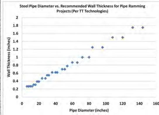
Figure 10. Minimum Wall Thickness Recommendations for Pipe Ramming (Courtesy of TT Technologies)
