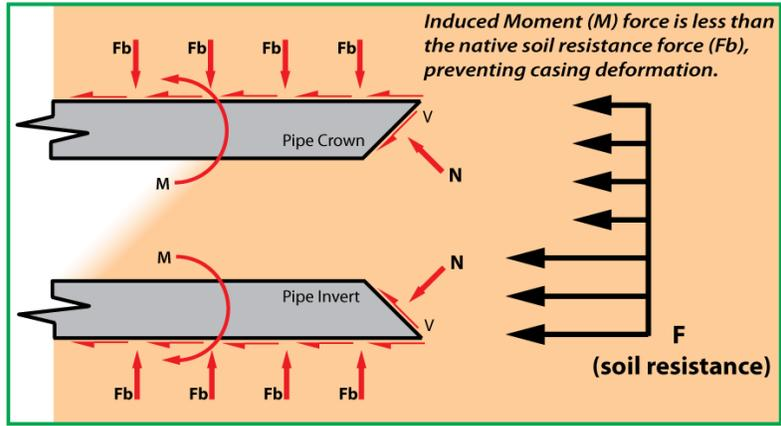
Figure 7. Force Diagram of Properly Designed Cutting Shoe
