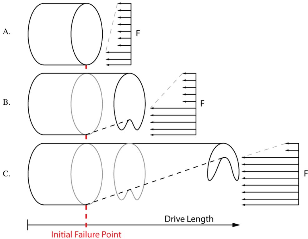
Figure 4. Illustration of Differential Stress on Leading Casing Pipe due to Dense Glacial Soils at Pipe Invert and Fill Soils at Pipe Crown
