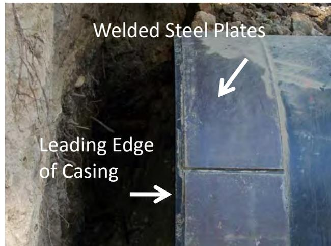
Figure 9. Failed Pipe Ram Cutting Shoe
