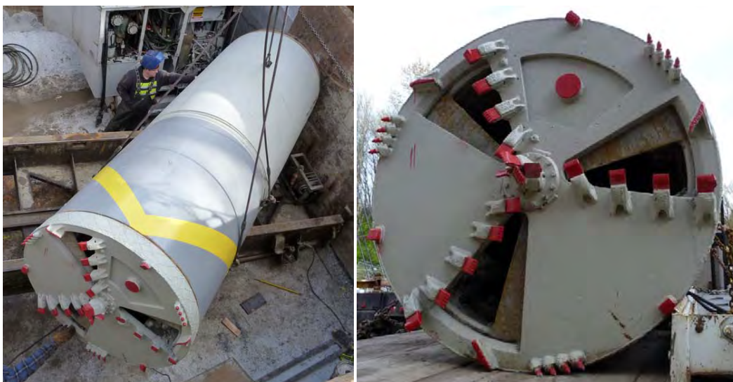
Figure 5. 60-inch Diameter Open Shield Pipe Jacking Machine Used on the Project.
