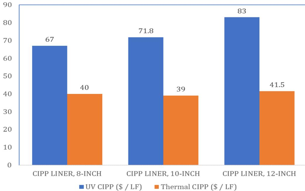
**Figure 6: UV and Thermal Cure CIPP Unit Cost Comparison**
