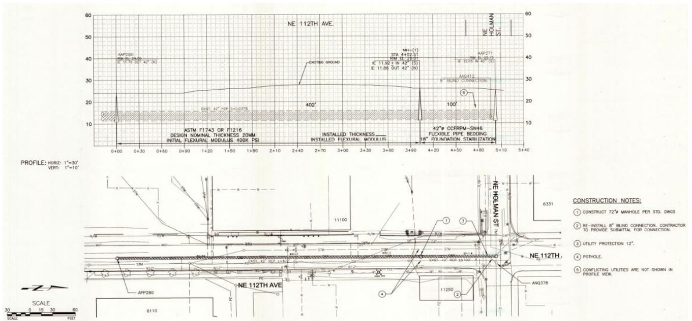
**Figure 2: Design or Replacement of the failed 42" pipe**
