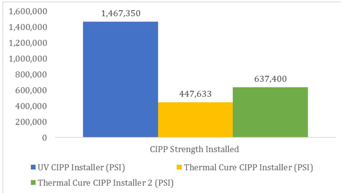
**Figure 8:** UV and Thermal Cure CIPP Flexural Modulus Comparison
