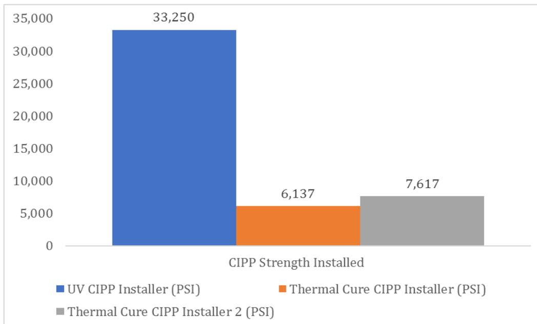
**Figure 7: UV and Thermal Cure CIPP Strength Comparison**
