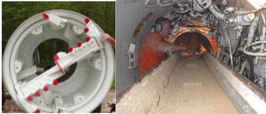
Figure 5 Open Shield Tunneling Machine Looking from Front (left) and from Inside (right)
